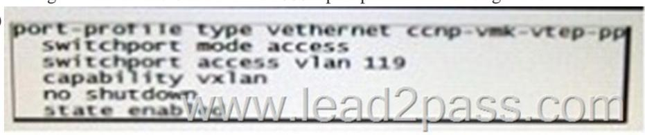
A. service-policy type qos output vmk-control B. vmware port-group C. system vlan 119 D. capability 13control E. switchport mode trunk F. mtu 9000 Answer: BCD
